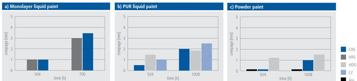
The neutral salt spray test shows that Gardo® Plus produces very good results when combined with a variety of paints and substrates.
